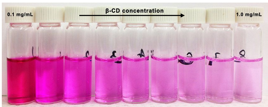
Figure S2. Phenolphthalein solutions with increasing β-CD concentration, where color faded from pink to colorless.
