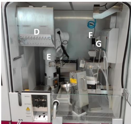
Figure S2 : Overview of the Compact SelecT platform. (A) Flask carousel incubator, (B) Plate incubator, (C) Media pumps, (D) Decappers, (E) Robot arm, (F) Pipette head and (G) IncuCyte live-cell analysis System .
