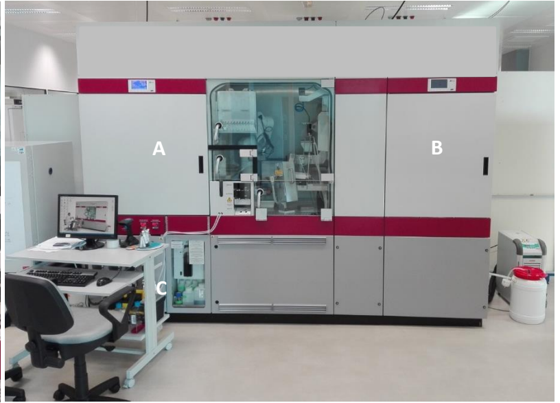
Figure S2 : Overview of the Compact SelecT platform. (A) Flask carousel incubator, (B) Plate incubator, (C) Media pumps, (D) Decappers, (E) Robot arm, (F) Pipette head and (G) IncuCyte live-cell analysis System .
