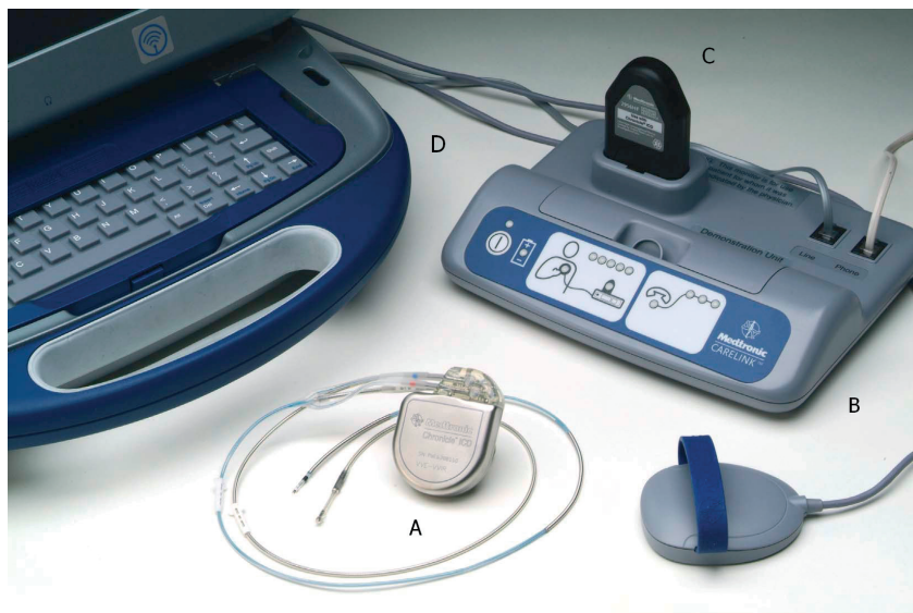
FIG. 2 The Chronicle ICD system includes the implantable device (A), a home monitor (B) that enables remote interrogation of the device and data transmission over standard telephone lines to a secure Web site. Absolute intracardiac pressure measured by the device are adjusted for barometric pressure captured by a time-synched external pressure reference (C) carried by the patient. The device can also be interrogated using a standard programmer (D).
