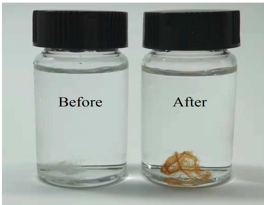
Figure S6. Morphology of Anti-AO before and after uranium adsorption.
