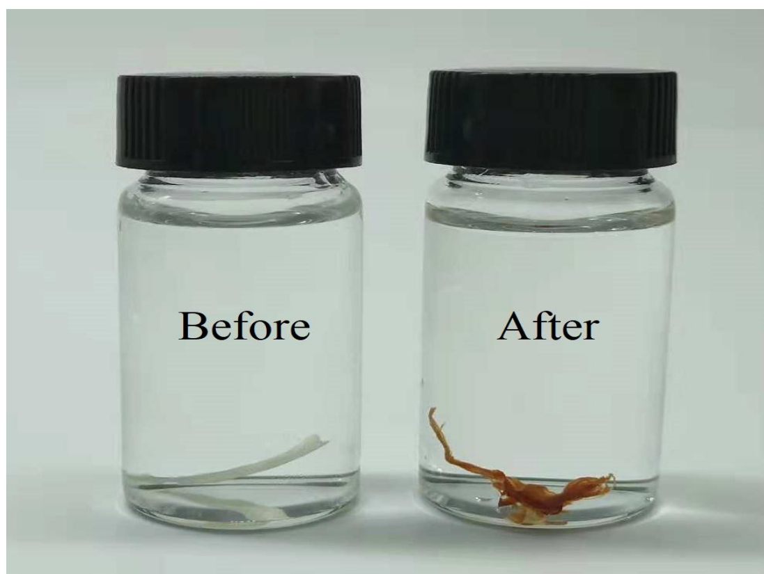
Figure S5. Morphology of Anti-PIDO before and after uranium loading.
