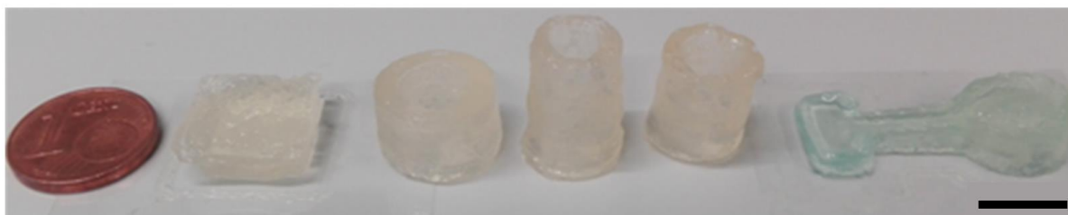
Figure S2. Examples of printed objects further highlighting the applicability of the in house-modified system for fabrication of 3D constructs. From left to right: one euro cent for comparison; half-cut and upside-down pyramid; cylinders of different diameters and heights; spoon-shaped objects. Scale bar: 10 mm.
