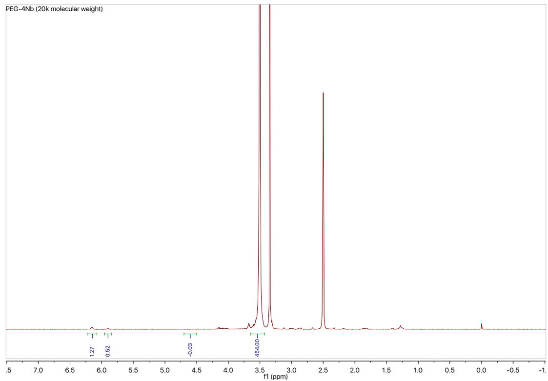
**Figure S3.**  $^1\text{H-NMR}$  of PEG-4Nb (20k molecular weight). Successful reaction is confirmed by  $^1\text{H-NMR}$  in  $\text{DMSO-d}_6$ : 400 MHz  $\delta$  6.20 to 5.86 (m, 2H; norbornene double-bond peaks),  $\delta$  3.65 to 3.40 (m, 454H; PEG backbone peak) and disappearance of the -OH peak at  $\delta$  4.60 to 4.50 (t, 1H). Modification was 90% by integration of norbornene peaks.
