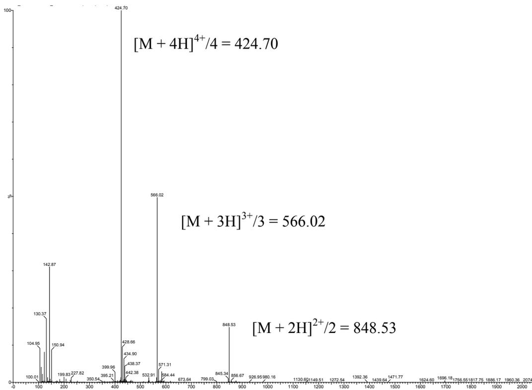
**Figure S5.** ESI-MS of synthesized DegXlink. Expected MW: 1695.98 g/mol. Observed MW:  $[M + 2H]^{2+}/2 = 848.53$ ;  $[M + 3H]^{3+}/3 = 566.02$ ;  $[M + 4H]^{4+}/4 = 424.70$ ;
