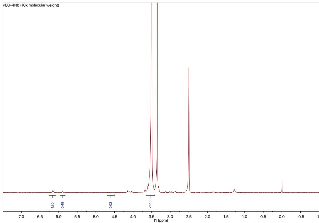
**Figure S2.**  $^1\text{H-NMR}$  of PEG-4Nb (10k molecular weight). Successful reaction was confirmed by  $^1\text{H-NMR}$  in DMSO- $d_6$ : 400 MHz  $\delta$  6.20 to 5.86 (m, 2H; norbornene double-bond peaks),  $\delta$  3.65 to 3.40 (m, 227H; PEG backbone peak) and disappearance of the -OH peak at  $\delta$  4.60 to 4.50 (t, 1H). Modification was 89% by integration of norbornene peaks.
