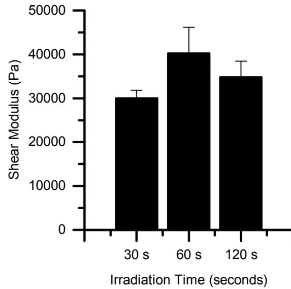
**Figure S7. The effects of irradiation time on the modulus of 20% w/w, 10 kDa PEG-4NB hydrogels.** Irradiating for 30 seconds or longer led to a roughly constant modulus, indicating that gel formation is essentially complete by 30 seconds. To ensure complete gel formation, 60 seconds of irradiation was selected for the studies presented in this manuscript.
