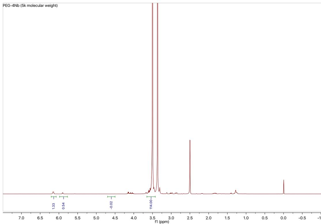
**Figure S1.**  $^1\text{H-NMR}$  of PEG-4Nb (5k molecular weight). Successful reaction was confirmed by  $^1\text{H-NMR}$  in DMSO- $d_6$ : 400 MHz  $\delta$  6.20 to 5.86 (m, 2H; norbornene double-bond peaks),  $\delta$  3.65 to 3.40 (m, 114H; PEG backbone peak) and disappearance of the -OH peak at  $\delta$  4.60 to 4.50 (t, 1H). Modification was 94% by integration of norbornene peaks.
