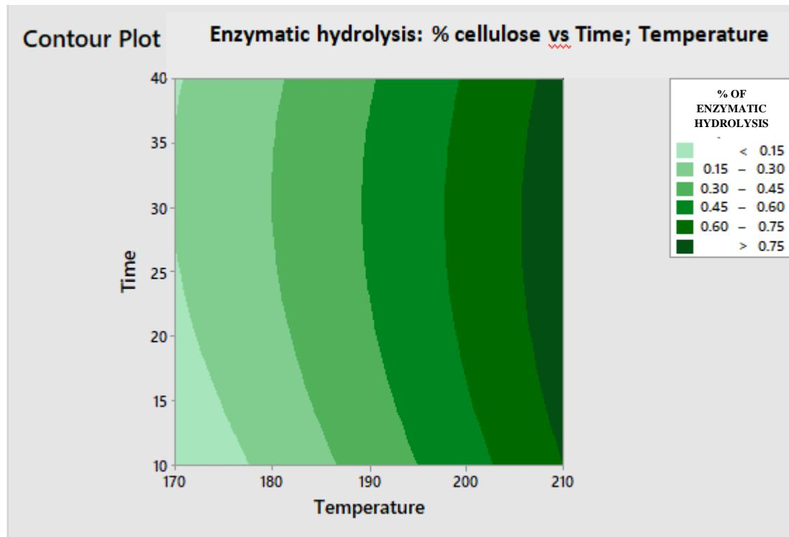
**Fig. S1.** Graphical response of the dependent variable (% of enzymatic hydrolysis) as a function of the two independent variables [temperature of SE (°C) and time of SE (minutes)].
