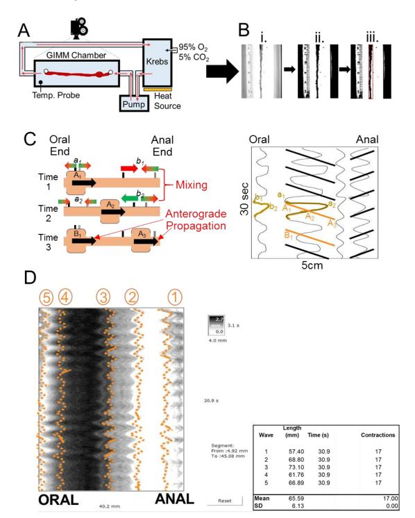
**GIMM instrument setup, data collection, and analysis**. A. GIMM design. A GI segment (dark red) is immobilized by two pins (white circles) in the GIMM chamber, which is filled with circulating,
