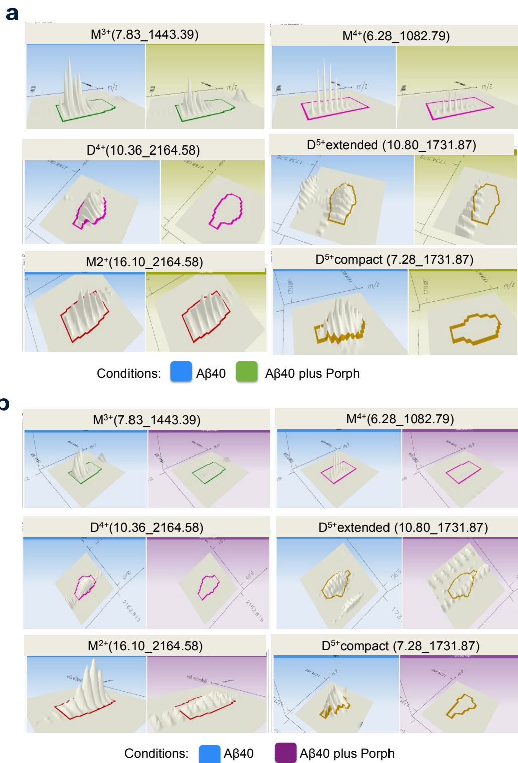
Fig. S6 3D montage m/z vs. drift time vs. intensity measured for a run of the “Aβ40” sample-class and a run of the “Aβ40 plus Porph” sample-class containing Zn-Porph (Aβ40:Zn-Porph, 1:1) at 5 \mu\text{M} (a), at 20 \mu\text{M} (b). On the 3D montage is shown the automated peak picking of the protonated monomers and dimers of Aβ40 assigned to the \text{M}^{3+} , \text{M}^{4+} , \text{D}^{4+} , \text{M}^{2+} and to the compact and extended conformations of \text{D}^{5+} based on the measured isotopic envelope and drift time (dt)
