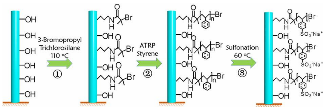
Supplementary Figure 1. Sulfonated poly(styrene) (SPS) grafting process.
