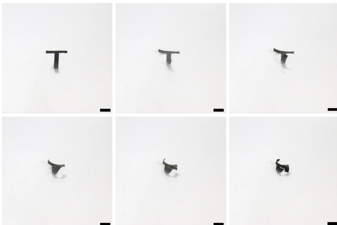
Supplementary Figure 24. The structure change process of T-like GO/PPy actuator under the stimulus of humidity (Scale bar: 1 cm).
