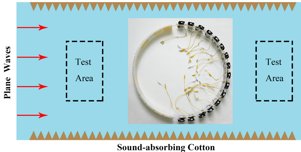
FIG. 4. Experimental implementation of the parity-time symmetric metasurface cloak.
