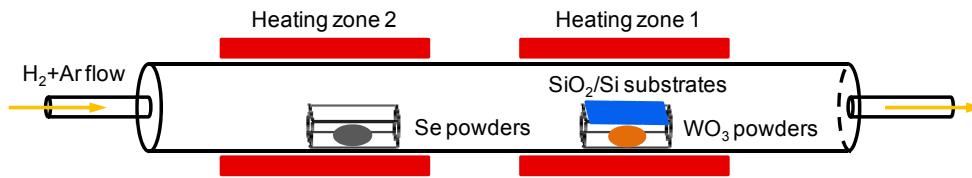
Fig. S1. Schematic illustration of the CVD system for WSe 2 nanostructures growth.
