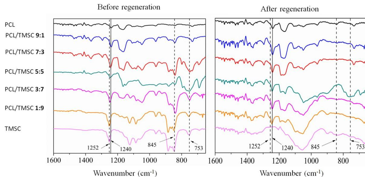
**Figure S3.** ATR-IR spectra of PCL/TMSC films for the region 650 – 1600  $\text{cm}^{-1}$ . The lines show the peaks assigned to TMSC/Cellulose (dotted, C-Si rocking vibrations at 1252, 845 and 753  $\text{cm}^{-1}$ ) and PCL (straight, asymmetric C-O-C stretching at 1240  $\text{cm}^{-1}$ ) before and after regeneration.
