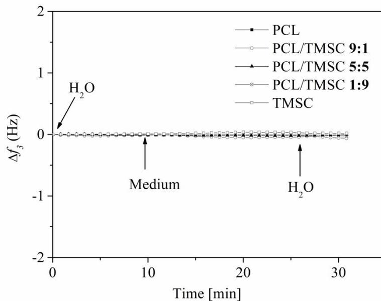
**Figure S4.** QCM-D frequency changes for the adsorption of the cell growth media EBM-2, Lonza, on PCL/TMSC surfaces after regeneration.
