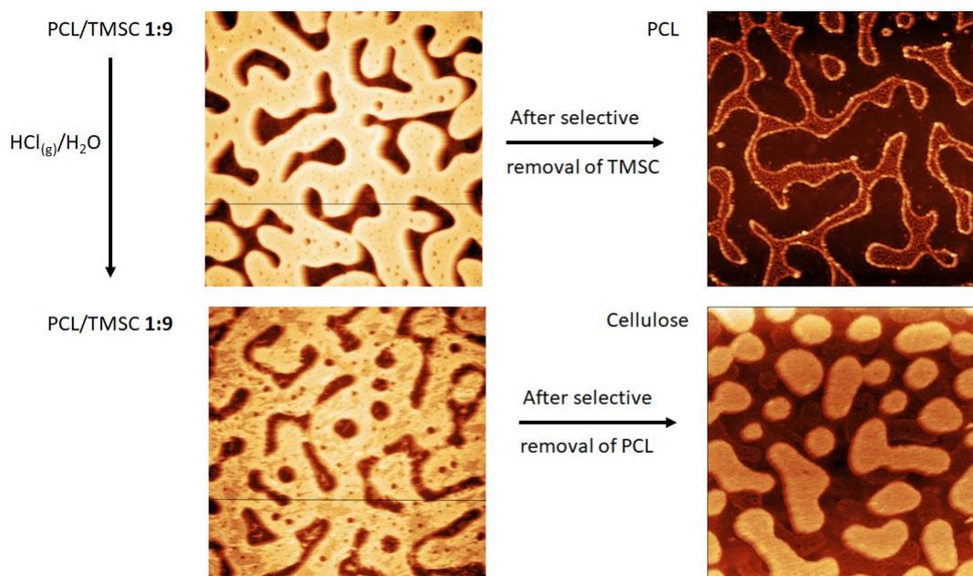
**Figure S1.** AFM topographical image ( $10 \times 10 \mu\text{m}^2$ ) of a PCL/TMSC film (top left) after the removal of TMSC with hexamethyldisiloxane (HMDSO) (top right) and a PCL/Cellulose film (bottom left) after the removal of PCL with chloroform (bottom right) (image size  $10 \mu\text{m} \times 10 \mu\text{m}$ ).
