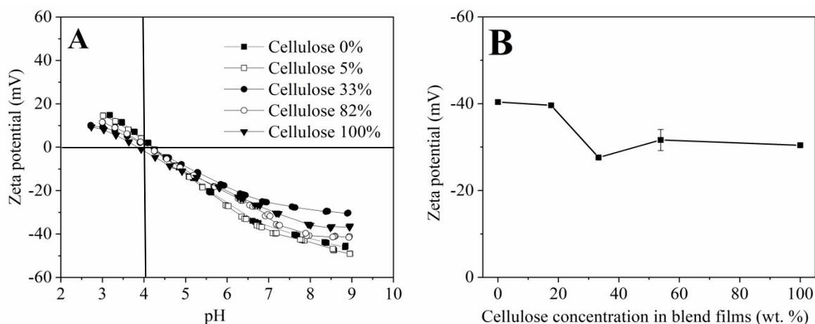
**Figure S5.** A) zeta potential of blend films containing increasing amounts of cellulose. B) zeta potential at pH 7.4.
