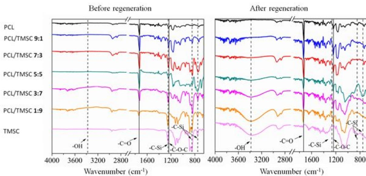
**Figure S2.** ATR-IR spectra of PCL/TMSC films, before and after regeneration with HCl vapors. The lines show the peaks assigned to the functional groups of either TMSC/Cellulose (dotted) or PCL (straight).
