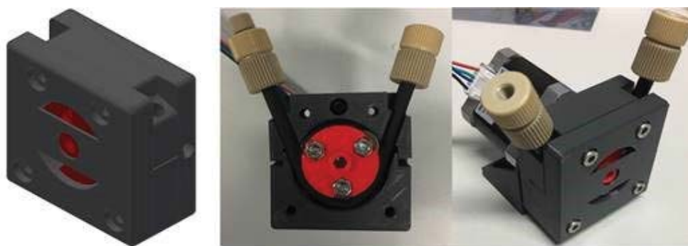
Figure S1: Peristaltic pump developed and produced in-house. Left: rendering of the pump design in Autodesk Inventor; Centre: internal structure of the pump also showing the IDEX tubing adapters, Right: assembled pump showing the NEMA17 motor in the back
