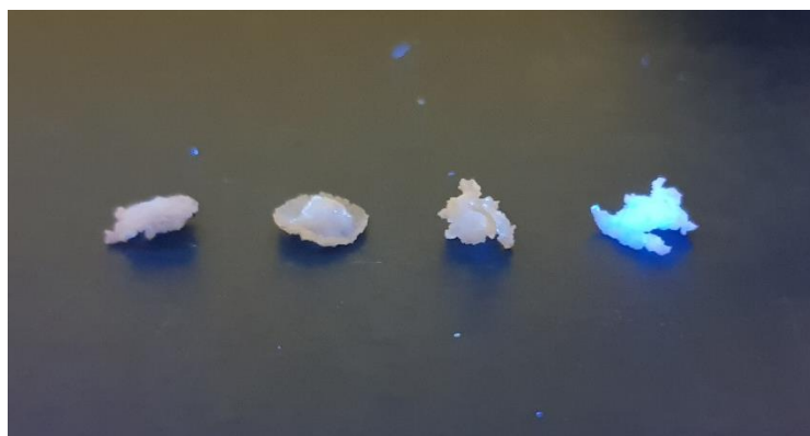
Figure S12. Photographs of fractured PHMA networks containing 0.02 mol% mechanophore under a UV hand lamp ( \lambda_{\text{exc}} = 365 \text{ nm} ). From left to right: PHMA 3 (containing terminal mechanophore), PHMA 4 (containing blended but not bound mechanophore), PHMA 5 (containing no mechanophore), PHMA 1 (containing mechanophore).
