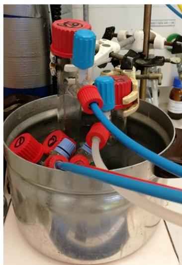
General Catalysis setup 4 reactions in one oil bath
