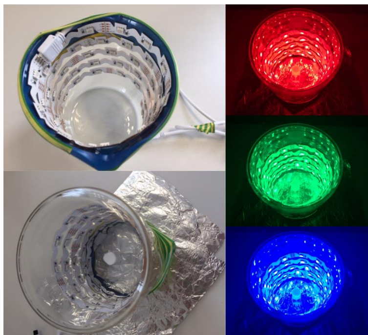
Figure S3: Setup for irradiation with visible light of 630 nm (red), 500 nm (green) or 452 nm (blue).
