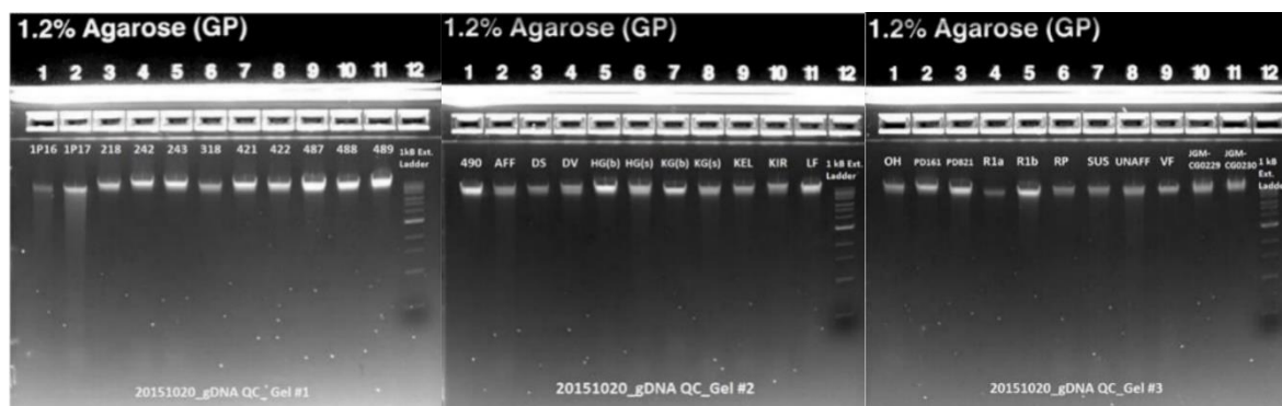
Supplementary Figure 2. Agarose gel electrophoresis of gDNA. DNA samples had a tight band with minimal smearing, therefore passing quality control.
