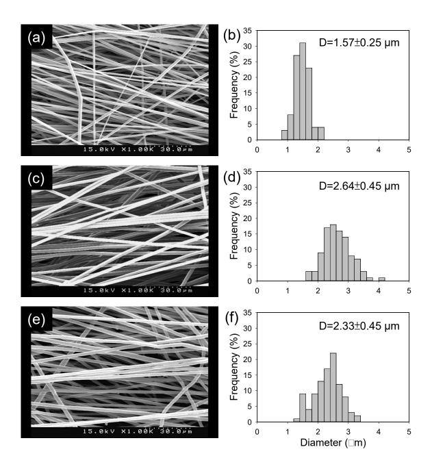
Supplementary Figure 1. SEM images of as spun PLA fibers (a), PEO/PLA blend fibers (c), and blend fibers with the PLA removal (e), and the corresponding distributions of fiber diameter (b, d, f). Note that 10% (w/v) PLA solution was used for preparing the as spun PLA fibers.
