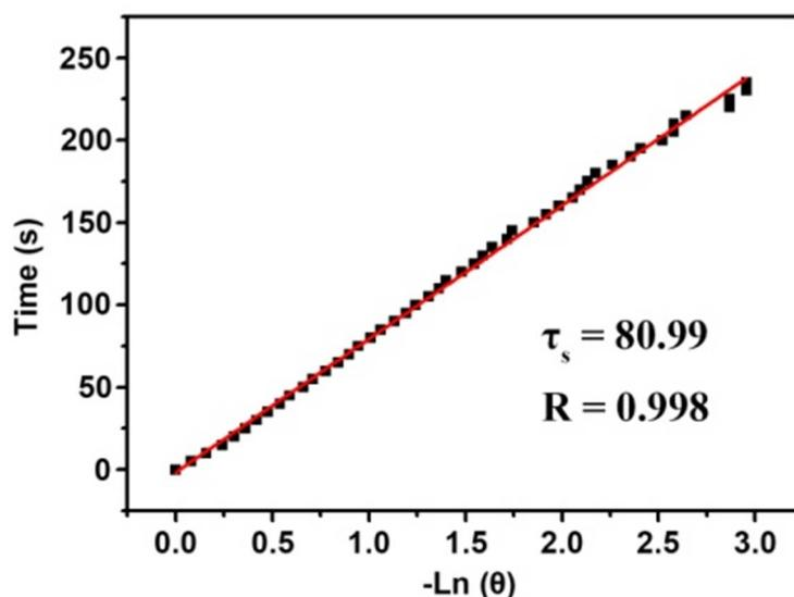
**Figure S6.** Time constant for heat transfer from the system ( $\tau_s$ ), calculated from the cooling period of the panel (Figure 3a).
