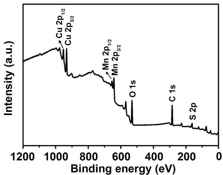
**Figure S2.** XPS survey spectrum of  $\text{Cu}_{2-x}\text{S}@\text{MnS}$  CSNPs.
