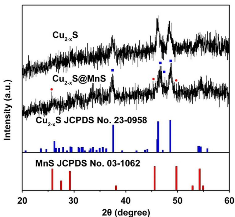
**Figure S1.** XRD pattern of as-prepared  $\text{Cu}_{2-x}\text{S}$  NPs and  $\text{Cu}_{2-x}\text{S}@\text{MnS}$  CSNPs. The blue and red dots above the black line denote monoclinic  $\text{Cu}_{2-x}\text{S}$  (JCPDS No. 23-0959) and hexagonal  $\text{MnS}$  (JCPDS No. 03-1062), respectively.
