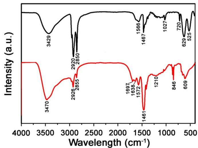
**Figure S5.** FTIR spectroscopy of Cu<sub>2-x</sub>S@MnS CSNPs before and after surface modification.
