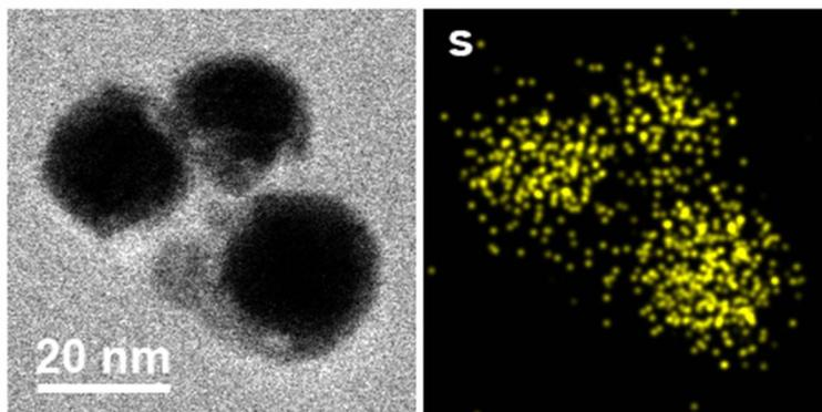
**Figure S3.** TEM elemental mapping with the sulphur window of  $\text{Cu}_{2-x}\text{S}@\text{MnS}$  CSNPs.
