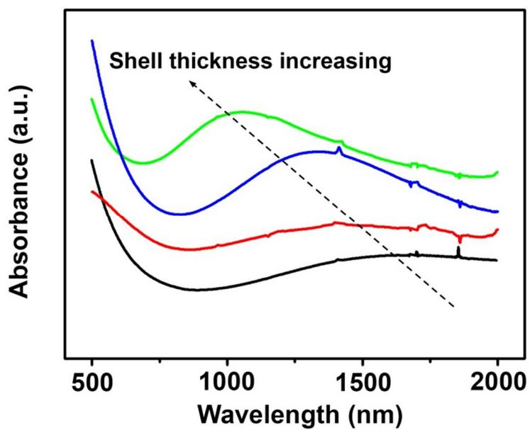
**Figure S4.** Vis-NIR absorption spectroscopy of the Cu<sub>2-x</sub>S@MnS CSNPs with different MnS shell thicknesses.
