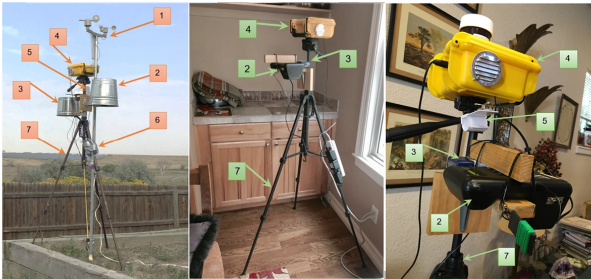
Figure S1. Outdoor instrument rig (Left) and Indoor Instrument rig (Middle and Right). [Legend for labels: 1 = Weather station; 2 = Dylos-1700 Monitor (outdoor instrument covered with metallic bucket); 3 = microAeth AE51 Aethalometer (outdoor instrument covered with metallic bucket); 4 = Y-pod; 5 = Ogawa NO 2 passive sampler; 6 = weather-protected electrical connection point; 7 = tripod stand.]
