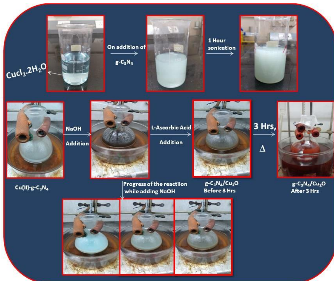
Figure S1: Pictorial representation of reaction with the sequence of color changes for the formation of g\text{-C}_3\text{N}_4/\text{Cu}_2\text{O} composite.
