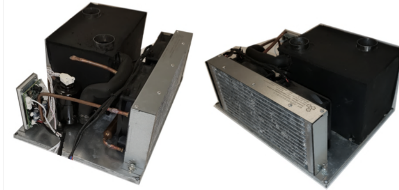
Figure S56. Pictures of the AC unit used as condenser to produce liquid water.
