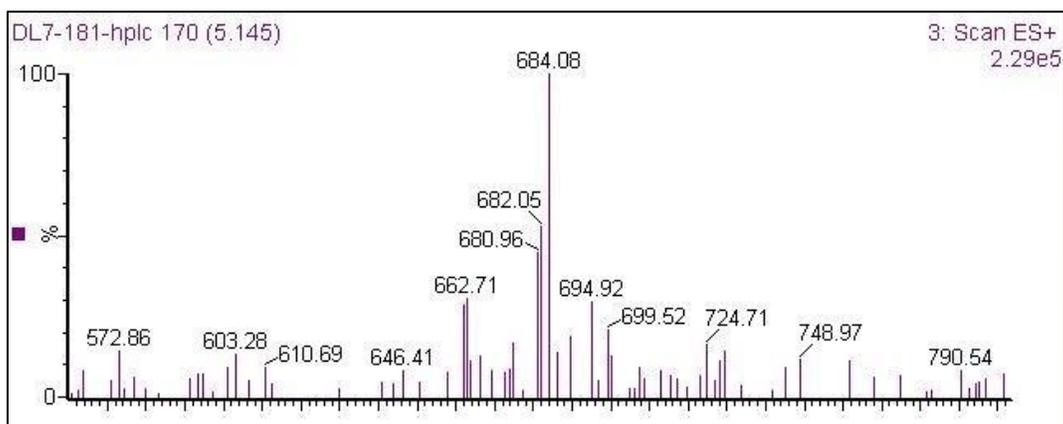
**Supplementary Figure 14.** LC-MS analysis for asymmetric hydrogenation of **5a'** using Duanphos for tri-hydrogenated intermediate.
