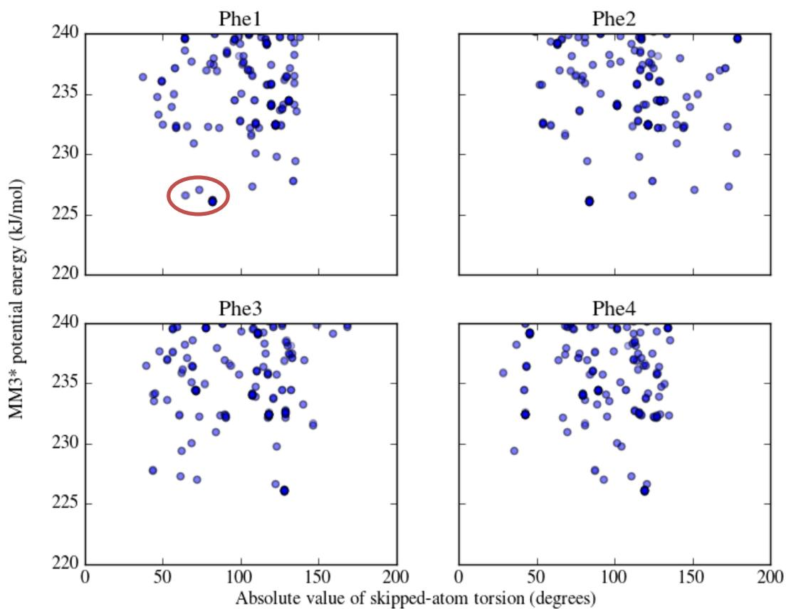
**Supplementary Figure 22.** Results from the Monte Carlo conformational search of the substrate. For skipped dihedral  $\Delta\text{Phe}_1$ , there is a cluster of low energy conformers with values of about  $57^\circ$ , the optimal geometry for catalyst binding.
