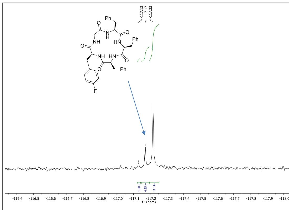
**Supplementary Figure 12.**  $^{19}\text{F}$ -NMR at  $t=15$  min for asymmetric hydrogenation of **5a'** using Duanphos
