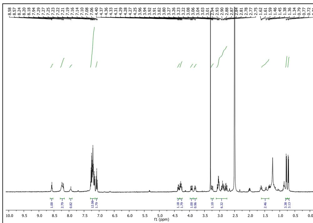
**Supplementary Figure 17.**  $^1\text{H-NMR}$  of cyclic pentapeptide **9a** after hydrogenation using (*R,R'*,*S,S'*)-Duanphos
