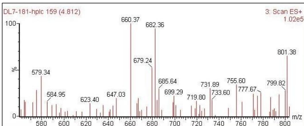
**Supplementary Figure 15.** LC-MS analysis for asymmetric hydrogenation of **5a'** using Duanphos for di-hydrogenated intermediate.
