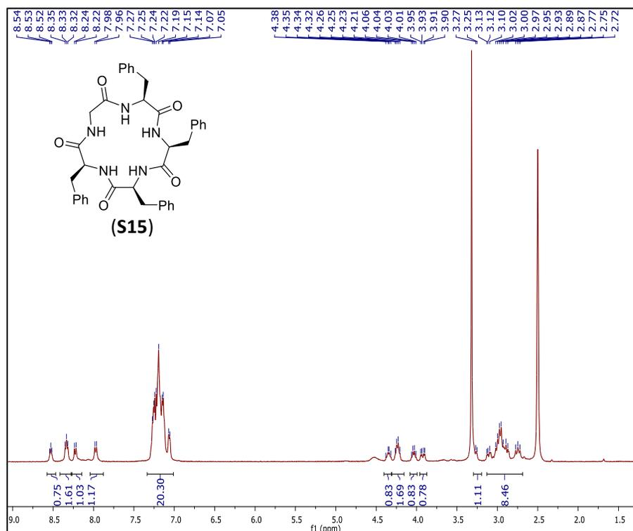
Supplementary Figure 7.  $^1\text{H-NMR}$  of cyclic pentapeptide **S15** made via SPPS
