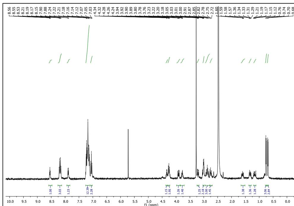
**Supplementary Figure 16.**  $^1\text{H}$ -NMR of cyclic pentapeptide **S19** made via SPPS
