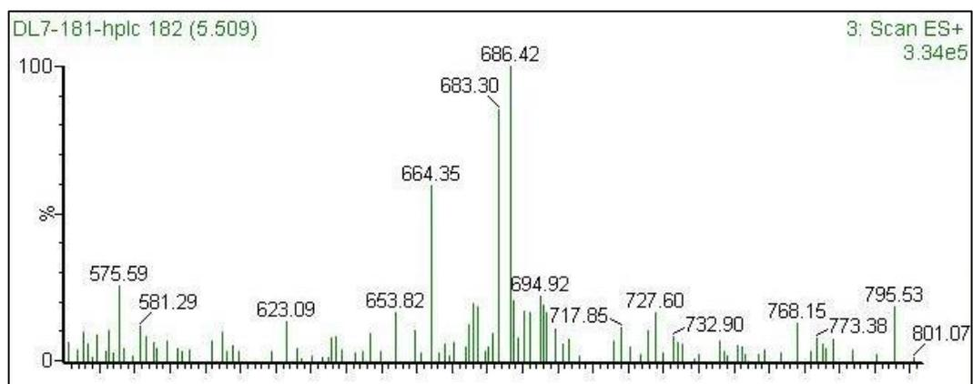
**Supplementary Figure 13.** LC-MS analysis for asymmetric hydrogenation of **5a'** using Duanphos for product formation.
