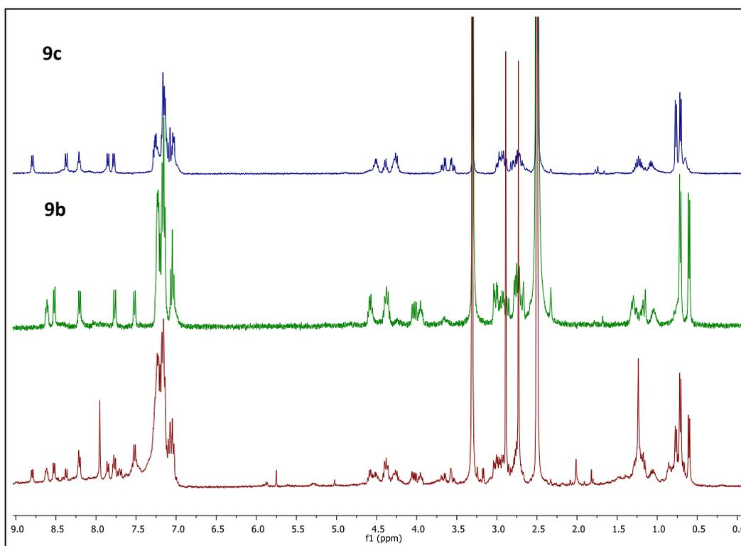
**Supplementary Figure 19.**  $^1\text{H}$ -NMR analysis for hydrogenation of **8** using dppp ligand. Blue spectrum represents authentic sample of **9c**, green spectrum represents authentic sample of **9b**, red spectrum represents spectrum of unpurified reaction mixture.
