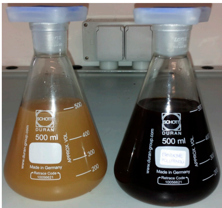
Figure S1. Pictures of unabsorbed fraction eluted with water (PAD428-FR1, left) and fraction eluted with water/ethanol (50/50) solution (PAD428-FR2, right).
