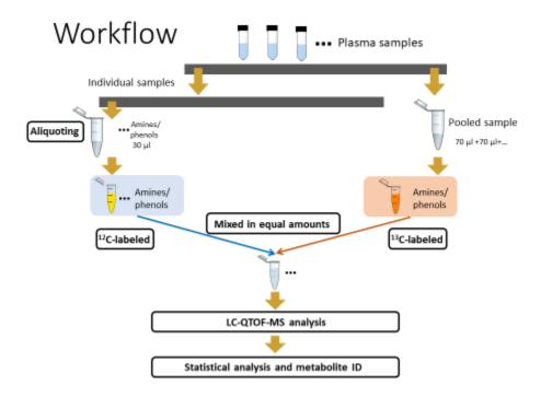
**Figure 1**. Workflow of the chemical isotope labeling/liquid chromatography—mass spectrometry method for analyzing the amine/phenol-containing submetabolome.
