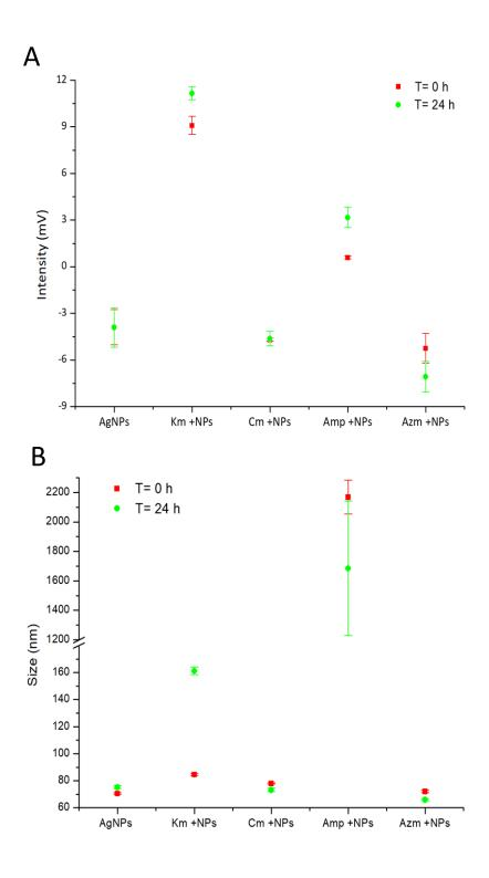
S3 Fig. DLS analysis of the combined AgNPs and antibiotic treatments at 0 (red) and after 24 hours of incubation (green). The charge (A) and size (B) of AgNPs are different for each antibiotic.
