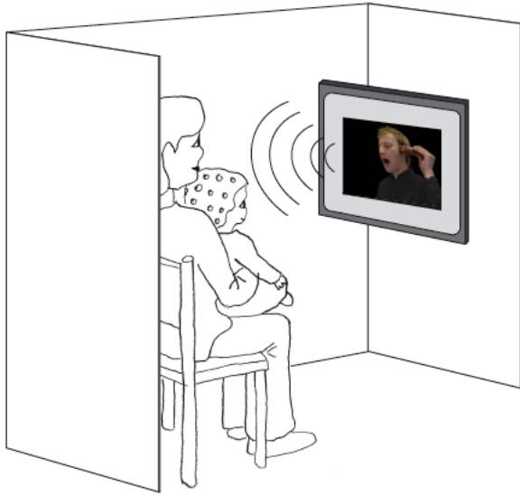
Fig. S2. Illustration of the infancy EEG set-up. During stimulus presentation infants sat on their parent's lab in a sound-attenuated electromagnetically-shielded room. Stimuli (Fig. S1) were flickered in infants' theta (4 Hz) and alpha frequency (6 Hz) on a 17-inch 60 Hz CRT monitor.
