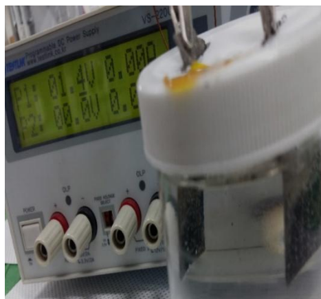
Supplementary Figure 26 | Photographic image of alkaline water splitting at 1.4 V in a two-electrode configuration for overall water splitting in 6M KOH solution, indicating the oxygen and hydrogen bubbles generation.
