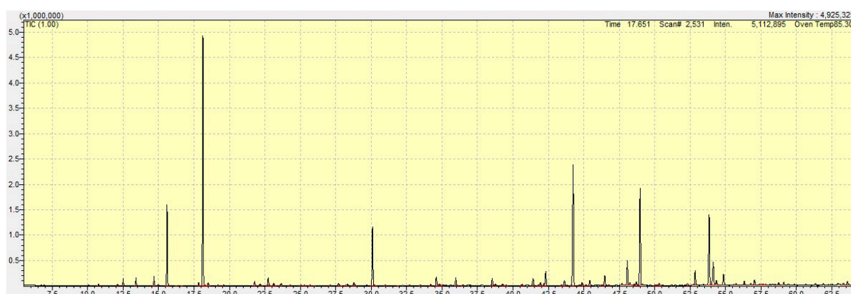
Figure S1. Total ion chromatogram of Piper arboricola leaves and stems essential oil.
