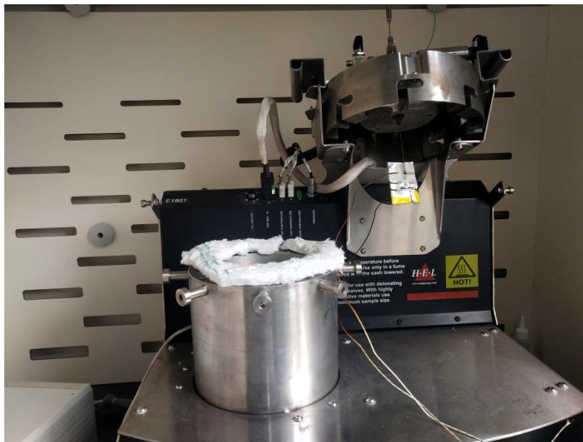
Figure S17. The reactor is the main component of the ARC test stand.
