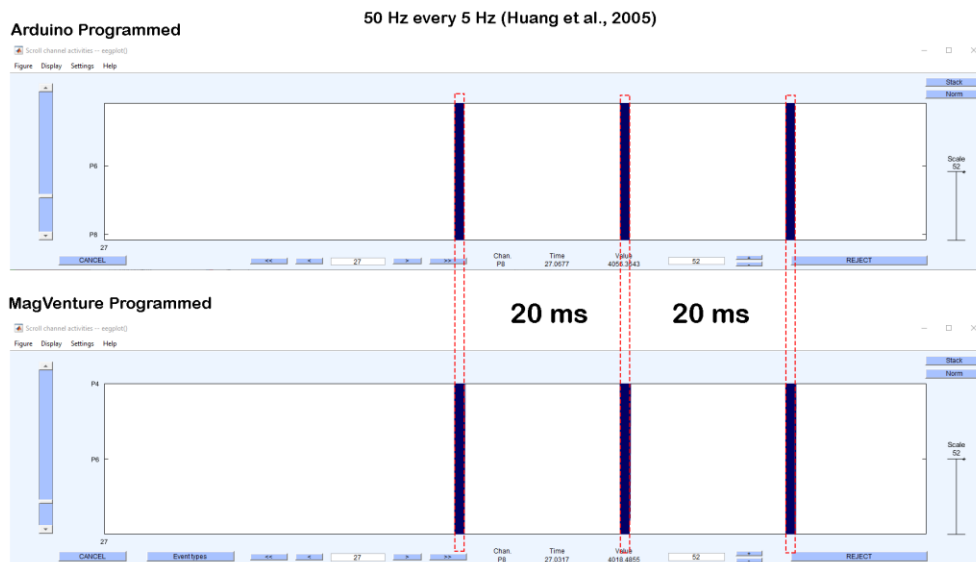
Figure S2. Comparison between MagVenture and Arduino programmed stimuli in electroencephalography (EEG) recording. (A) Inter-burst interval (5 Hz / 200 ms) and (B) Intra-burst interval (50 Hz / 20 ms). Red dotted boxes were drawn to illustrate how precisely pulses match.
