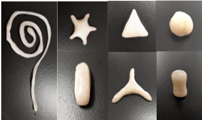
Figure S2. The ACP/PAA/CS hydrogel manipulated into various shapes.
