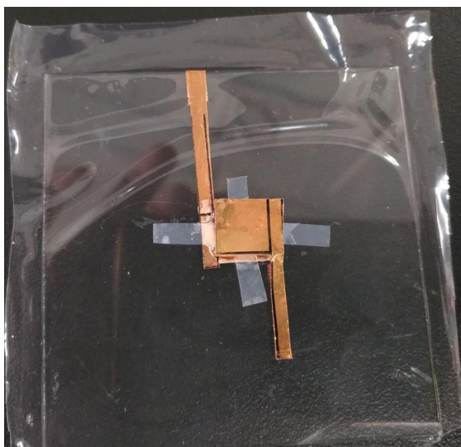
Figure S11. The dielectric layer of capacitive-pressure sensor.
