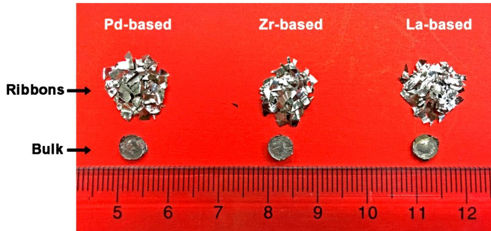
Fig. S3. Top views of the three metallic glass ribbons and the corresponding BMGs fabricated by the ultrasonic vibration method. (Photo credits: Dr. J. Ma, Shenzhen University)
