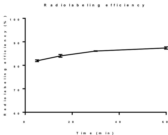
**Figure S3.** Radiolabeling efficiency of single-stranded DNA with Zr-89.
