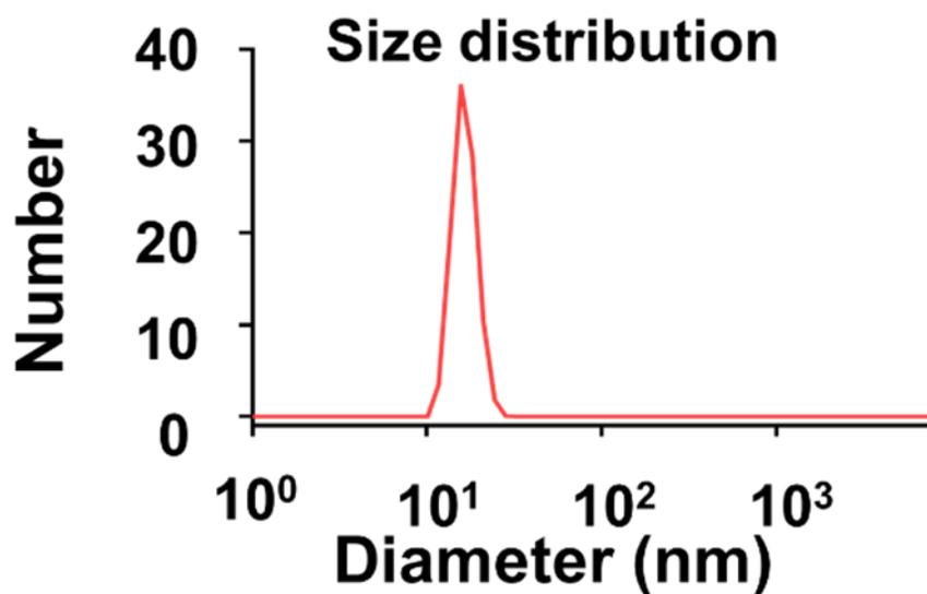
**Figure S2.** Dynamic light scattering measurement of FNA.
