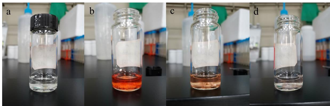
Supplementary Fig. 19 Qualitative test of formaldehyde by phloroglucinol. Electrolyte after the electrochemical glycerol anodic oxidation with (a) and without (b-d) phloroglucinol. The electrolyte rapidly turns orange when phloroglucinol was added and then quickly shallowed, indicating the presence of formaldehyde.
