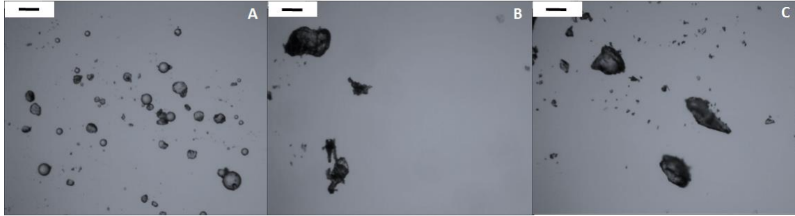
Figure S1. Light microscope images of (A) PMMA, (B) CS and (C) CSMCC particles. Magnification 10X. Scale bar 84.46 \mu\text{m} .
