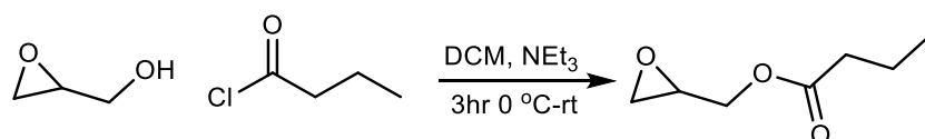
Supplementary Figure 1. Synthetic pathway of glycidyl butyrate from glycidol and butyryl chloride.
