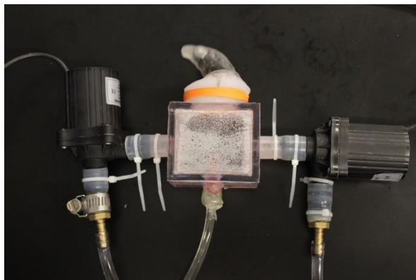
Figure S8. Embolism test set-up. Pumping water at physiological frequencies f = 1\text{Hz} . Measuring pressure within the idealized left atrium. Reservoir sits \sim 15'' below left atrium chamber.
