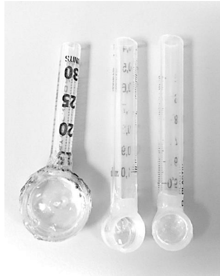
Figure S1: Customised sample holders of two sizes for imaging oviduct tissue samples. The tissue samples were pinned on the silicone elastomer surface with the UVJ mucosal surface and the SST orifices exposed.
