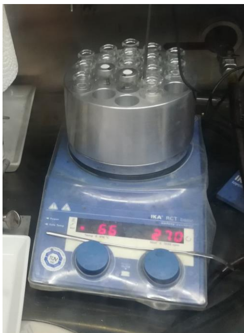
Figure S3. Picture of the set-up used for kinetic analysis with air sensitive samples in an argon-filled glove box.
