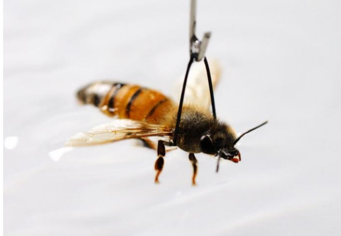
Fig. S6. Motion constrainer. A thin metal wire was bent into a fork shape to constrain a honeybee from wandering around. The constrainer did not interfere with the wing motion, and it did not constrain the body motion vertical to the water surface.
