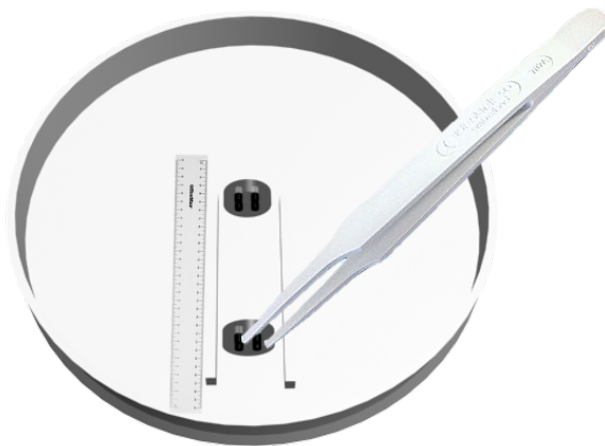
Fig. S5. Measurement of the attraction range of panels parallel to the disk axis on a vertical vibrational shaker: We fix one panel in the center of the sample cell and place the pairing panel with the right configuration at a designated distance in a guard rail (white lines) by a pair of plastic tweezers. After released by the tweezers, the panel either directly binds to the fixed panel or jostles around. We repeat each experiment 40 – 50 times and take the distance as the attraction range when in at least 80% of trials, the free panel is directed to bind.
