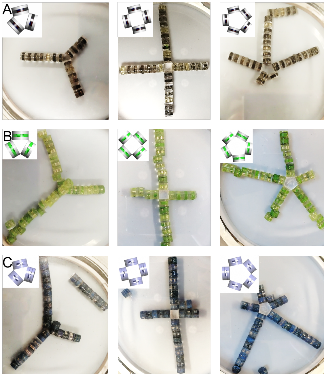
Fig. S6. Branched polymer formed by Black (A), Green (B) and Blue panels (C) with three (left column), four (middle column) and five branches (right column) from structured seeds shown in the insets.
