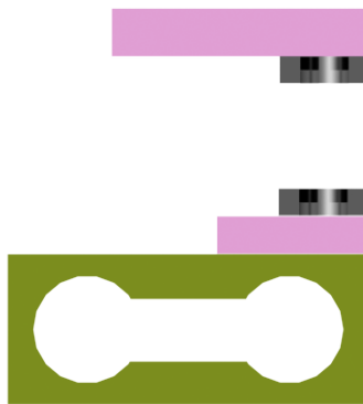
Fig. S4. Force measurement setup: We measure the magnetic interaction between two matching panels at the optimal pairing orientation on a single point load cell connected to a computer by a USB load cell interface and accurately control the surface-surface distance between panels with a motor and a micrometer mounted together.
