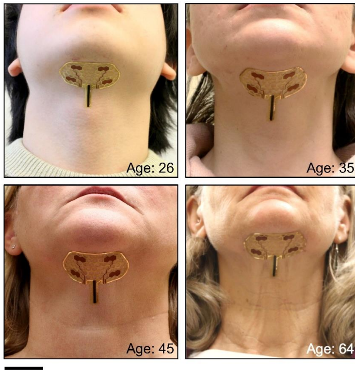
Fig. S1. Sensor patch adhered to the human submental skin of different ages. Photos of the sensor patch placed on human subjects of different ages (26~64). The scale bar is 3.5 cm. Photo Credit: Min Ku Kim, Purdue University, West Lafayette.
