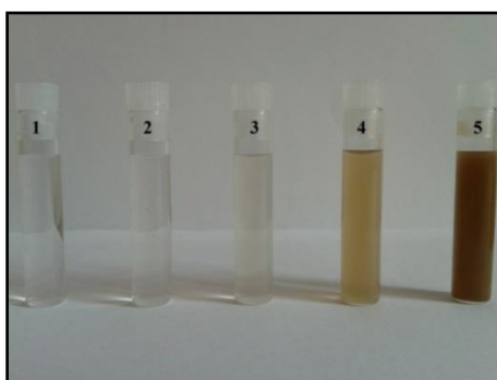
Figure S4. Optical image of 5 batches of liposomal dispersions ordered from left to right with respect to the volume of SPIONs dispersion used in the synthesis: 1. 0 \mu\text{L} (bare liposomes) 2. 10 \mu\text{L} 3. 50 \mu\text{L} 4. 250 \mu\text{L} 5. 1000 \mu\text{L} .
