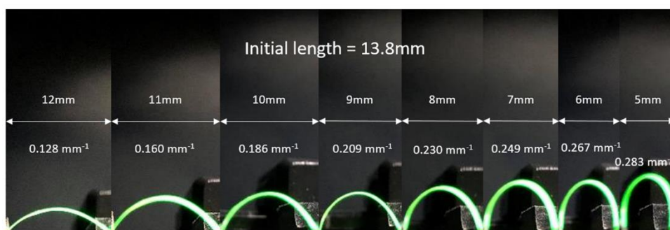
Figure S5. Optical photos of PQD papers under different bending curvatures.
