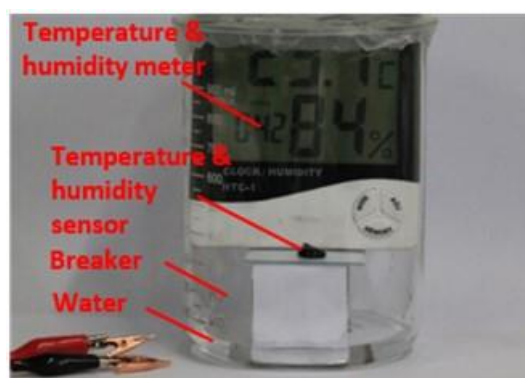
Figure S8. An experimental setup to monitor changes in humidity and temperature.
