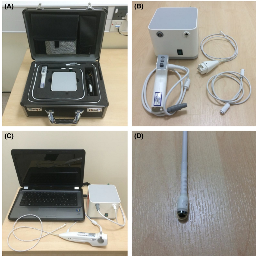
Figure 1. The EG ScanTM II system. (A) the portable case with four main parts; (B) the image processor (top left), disposable probe (top right), air tube (bottom right) and hand-held controller (bottom left); (C) the system connected and ready for use; (D) close view of the capsule probe tip. (Reproduced with permission from Sami SS, et al. Copyright John Wiley and Sons).
