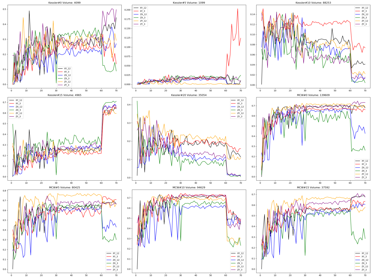
Figure 1: Test accuracy of nine samples in each of six different paths across different epochs of our model. We see no one path is consistently best.
